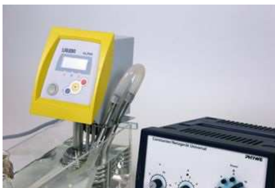
Fig. 2: External circulation set 08493-02 for water circulation.
